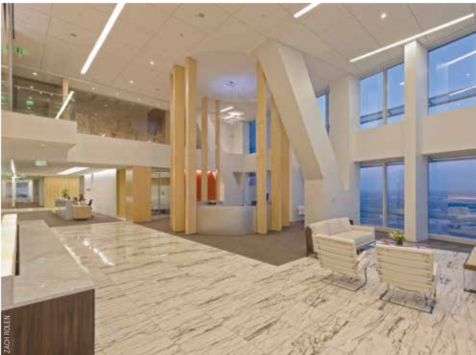
The space on floors 37 and 38, just beneath the sky-garden level, includes a two-level loft space that highlights the angled columns that shift inward to accommodate the sky garden above.
